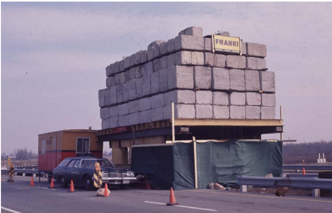
Figure 25. Load Testing a 49 m Floating Instrumented Steel Pipe Pile Preloaded by Downdrag over 10 years, Berthierville, 1980.
