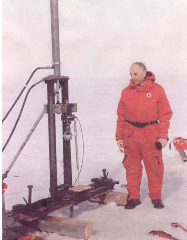
Figure 11. Branko Ladanyi Testing the Strength of Sea Ice Cover in Newfoundland, 1990
